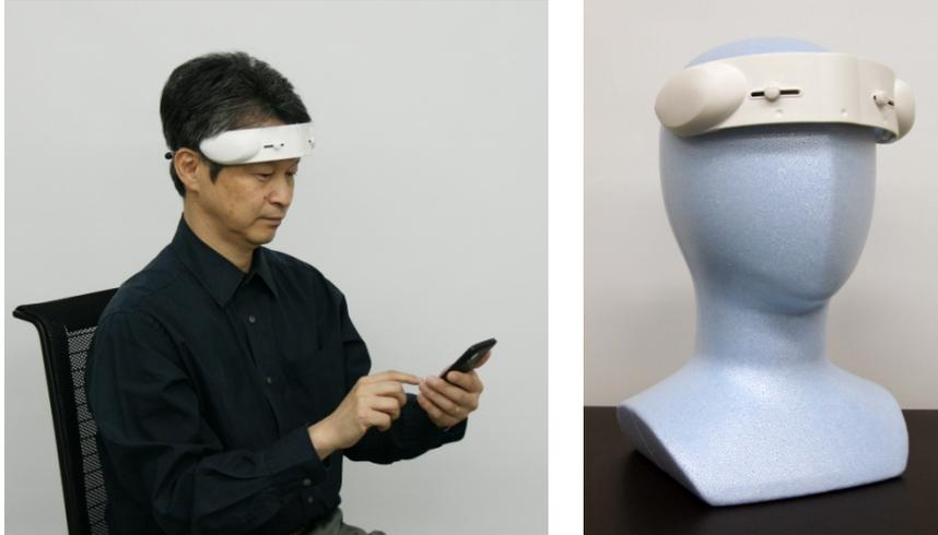
**Portable Brain Activity Measurement Device (Prototype)**
