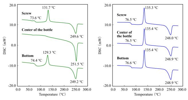
Figure 4 DSC curves of PET bottle for 1st heating
