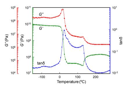
Figure 2 Viscoelastic spectrum of Carbon fiber reinforced epoxy prepreg (1st heating) Frequency: 1Hz
