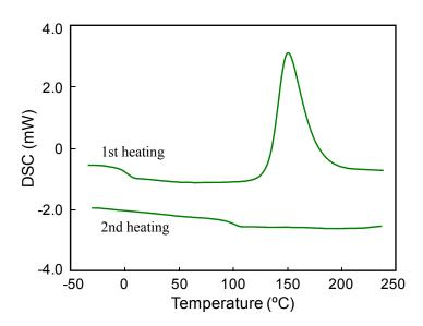
Figure 5 DSC curves of Carbon fiber reinforced epoxy prepreg Heating rate: 10°C/min
