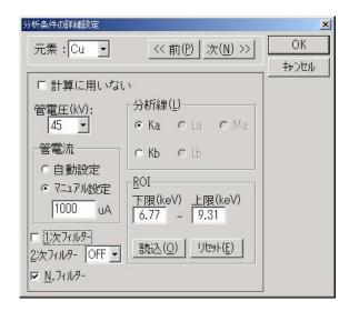
9. Input as shown in the window below and click on Next. Input as shown on the left when the thickness is less than 10 um and as on the right when the thickness is 10 um or greater.
