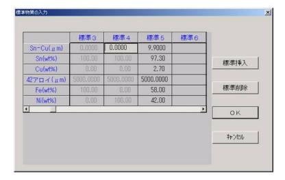
12. Including the items you just registered, numbers of the standard sample that should be measured are displayed as shown in the figure below. Exit after you have measured the concerned standards samples. Save the conditions. Default is Sn infinite in no. 1, Cu infinite in no. 2, Fe infinite in no. 3, Ni infinite in no. 4, and newly registered standard samples in and after no. 5.
