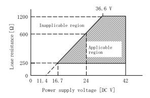
A minimum load resistance of  $250\,\Omega$  shall be required to communicate by connecting to communicator.
