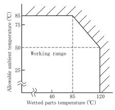
Fig.2 Wetted parts temperature and allowable ambient temperature
