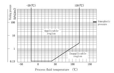
Fig.3 Working pressure and process fluid temperature
