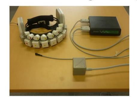
A digitizer (PATRIOT™) provided real-time measurements of position (X, Y and Z Cartesian coordinates) and orientation (azimuth, elevation and roll). X, Y and Z coordinates corresponding to the 16 channels, nasion, inion, Cz, and preauricular points were used as input data for the individual spatial analysis script running on Matlab (<a href="http://www.jichi.ac.jp/brainlab/index\_de.html">http://www.jichi.ac.jp/brainlab/index\_de.html</a>)
