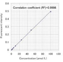
Hitachi's unique high-efficiency diffraction grating and low-noise detection system allow for measurement of very low concentrations.
