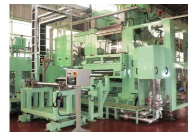
Roll press equipment used in the raw material process of LiB manufacturing Hitachi Power Solutions Co., Ltd.
