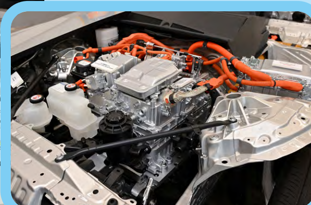
Fuel cell mounted in the second-generation MIRAI, achieving both high output and downsizing
