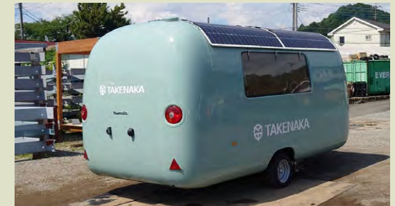
Off-grid mobile house. Even in locations without developed electric or communication infrastructure, independent power operation is possible through solar panels, storage batteries, and control devices, as well as satellite internet (Starlink).
