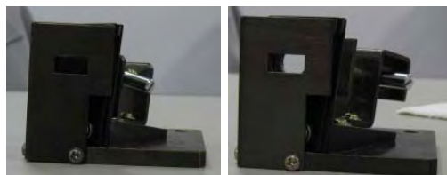
Figure 3 Appearance from the excitation light entrance (Left) Standard product, (Right) With a transmission hole
