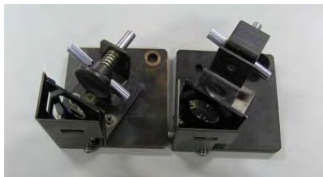
Figure 2 Appearance of solid sample holder (Left) Standard product, (Right) With a transmission hole
