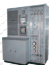
Model KLA-2 Column (40 \mu m particle) Analysis time 22 hrs.
