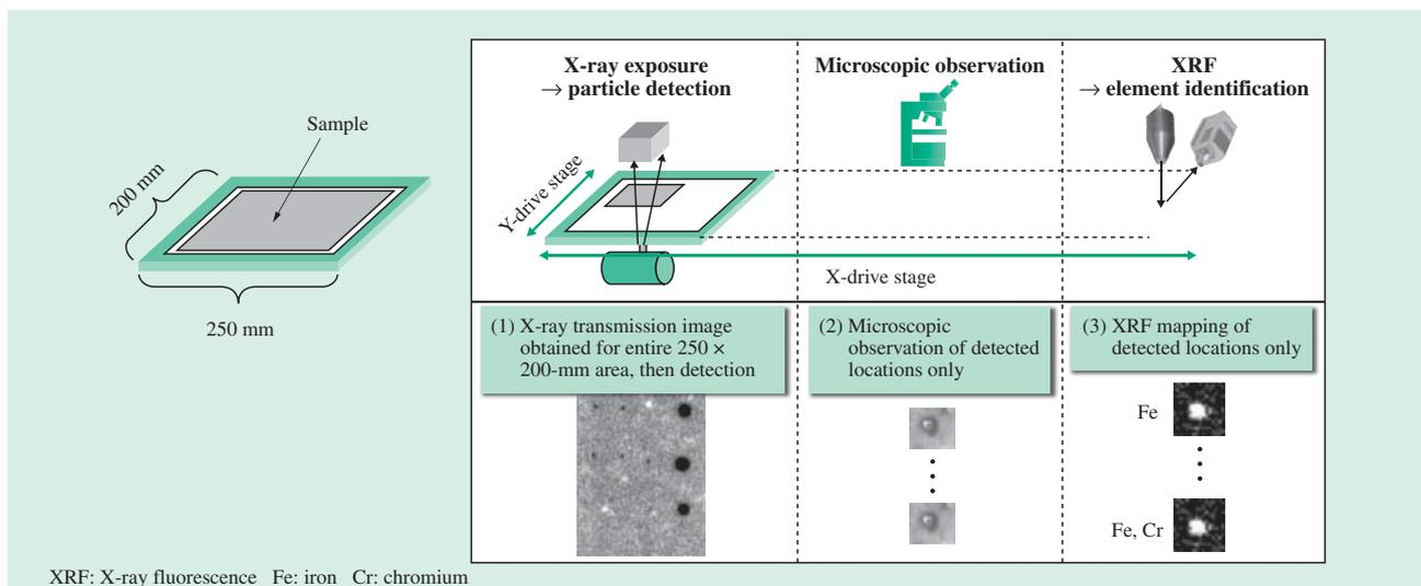
Fig. 2—Sequence of Steps in EA8000 Measurement.
