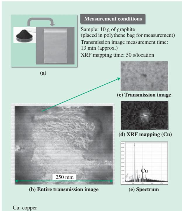
Fig. 4—Example Analysis of Carbon-based Powder Sample. Carbon-based powder can be measured with just simple sample preparation.
