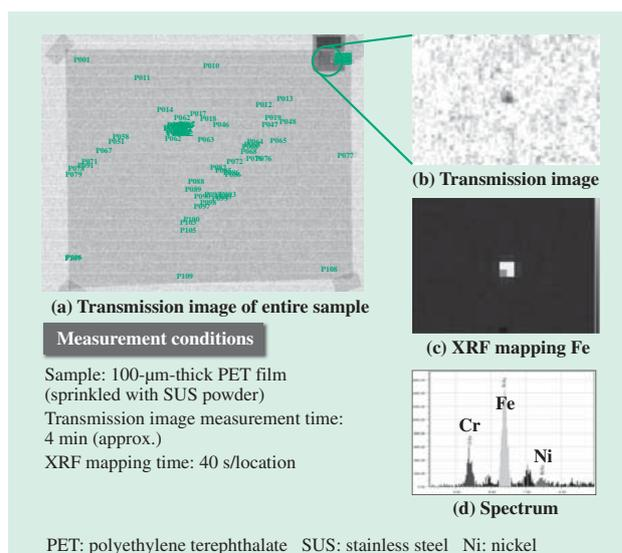
Fig. 6—Defect Analysis Sample for Analysis of Separator. (a) shows the full transmission image of the sample sprinkled with SUS powder, and (b), (c), and (d) show the analysis results for a particle of known size.
