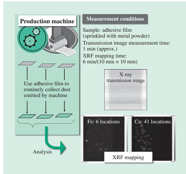
Fig. 5—Example Analysis of Sample for Dust Emitted by Production Machinery or Other Sources.
