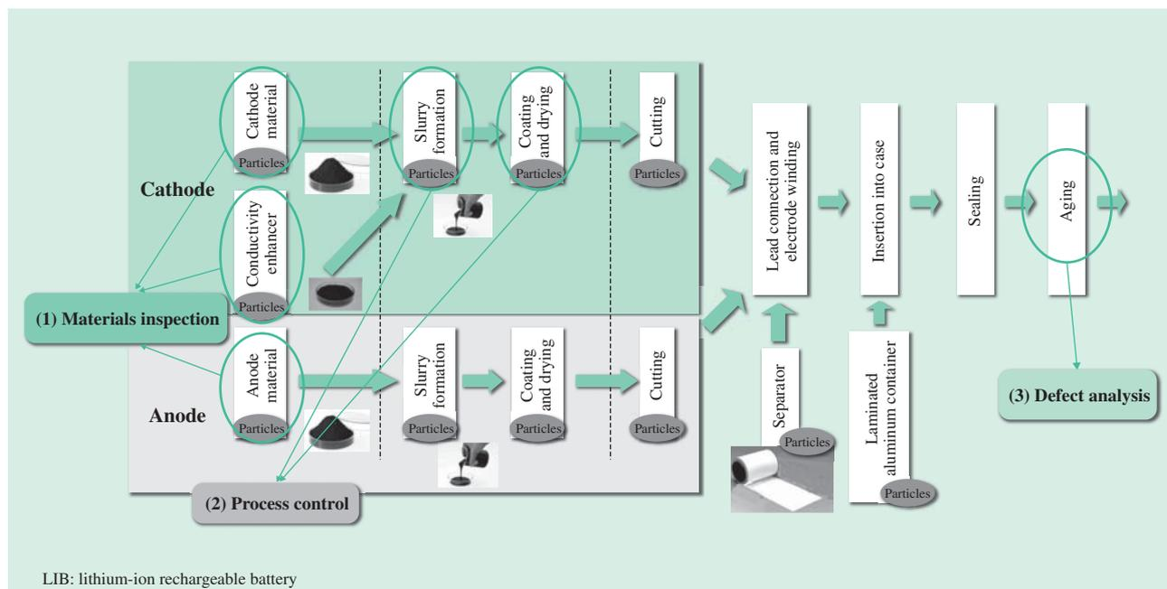
Fig. 3—LIB Manufacturing and Suitable Applications for EA8000 Analysis. There are applications for the EA8000 at various stages in the LIB manufacturing process.
