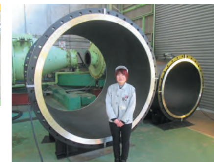
大口径電磁流量計実流試験装置 Large diameter electromagnetic flowmeter test facility
