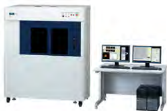
An X-ray particle analyzer helps to improve the production yield and reliability of lithium-ion batteries and fuel cells.
