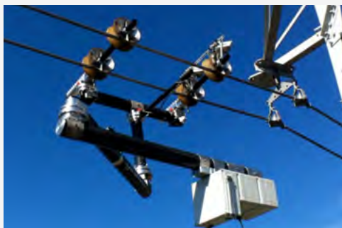
Expliner high-voltage transmission line inspection robot A self-propelled robot that moves along high-voltage overhead transmission lines to examine their external surface conditions and measure their outer diameter
