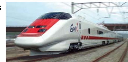
East-I, electric and track inspection train for shinkansen (Source: JR East Japan Railway Company)
