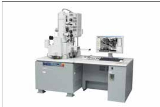
Field Emission Scanning Electron Microscope, SU8000
