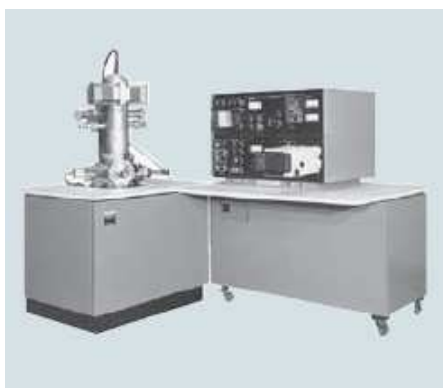
Hitachi Pioneered Development of the World's First Practical FE-SEM: the HFS-2 Model (Launched 1972)
