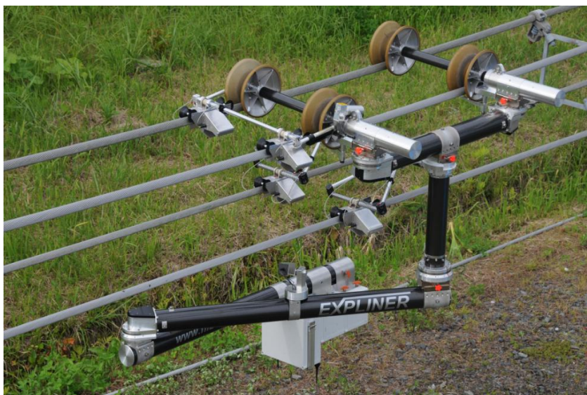
Overhead High-Voltage Transmission Line Inspection Robot Expliner
