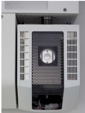
New heating furnace with view port
