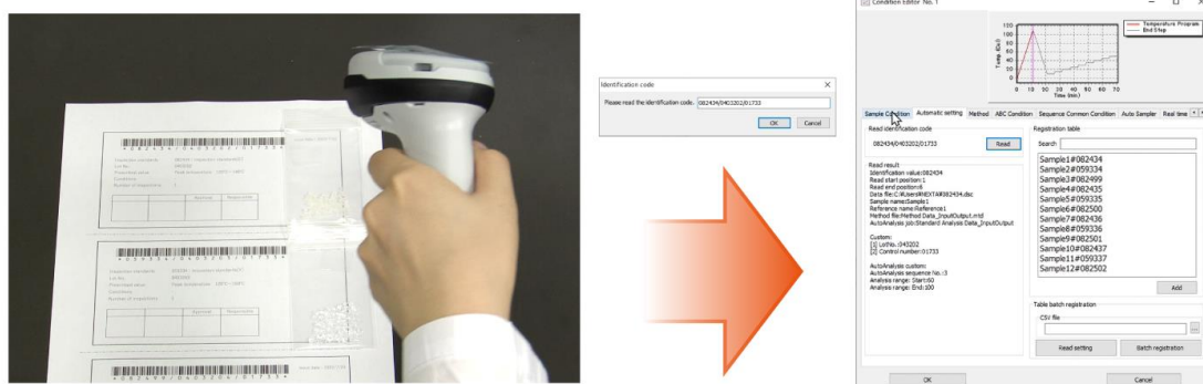
[Automatic entry of measurement conditions using a barcode reader, and the software screen after automatic entry]
