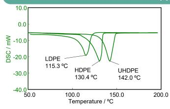
A series of commercial PEs were run on the DSC7000X using aluminum open pans. Samples were heated at 10 °C/min. Only the second heat is shown, While there is some variation in each grade, the low-density and high-density samples used are representative of grades 2 and 4, with LDPE melting at 115 and HDPE at 142 °C. As you can see, the materials are quite distinct in the DSC. In addition, we ran a medium density polyethylene. As expected, it falls directly in between the two.
