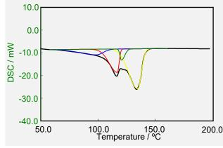
The above thermogram shows a mixture of four grades of PE One can easily seen the change from the HDPE peak. If one needs to estimate the components of the mixture, one can use the peak separation software to deconvolve the curve. One can then measure the component peaks and estimate their relative contribution.
