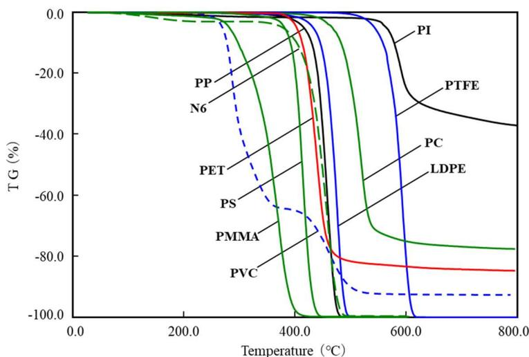
Figure 2 TG curves for each polymers in N<sub>2</sub>
