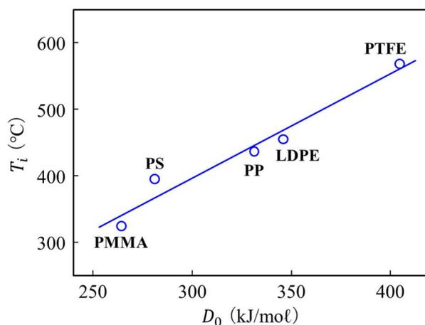
Figure 4 Relationship between  $T_i$  and  $D_0$  for PMMA, PS, PP, LDPE and PTFE
