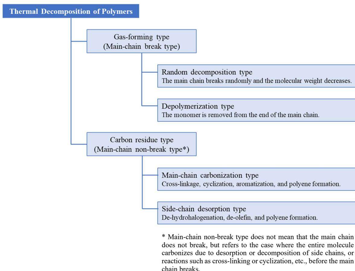
Figure 3 Classification of thermal decomposition patterns<sup>6)</sup>
