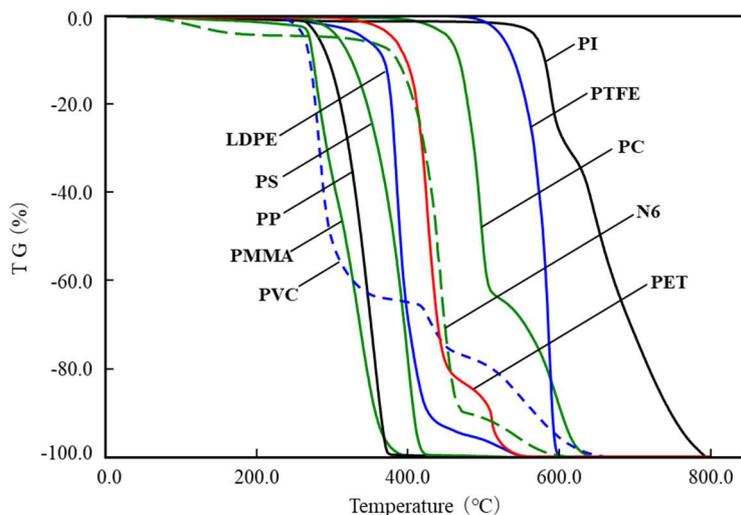
Figure 1 TG curves for each polymers in Air
