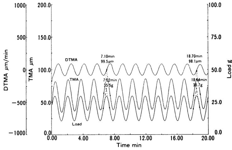
Figure 4 TMA/SS measurement results for LDPE film
