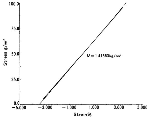
Figure 2 Stress-Strain graph for spring
