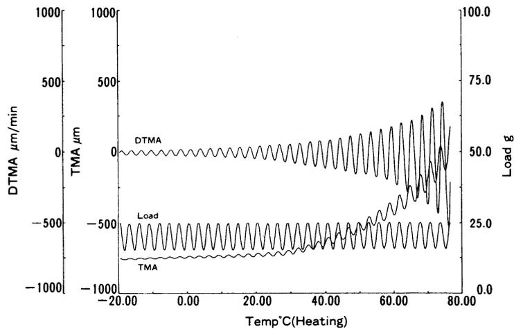
Figure 7 TMA/SS measurement results for LDPE film
