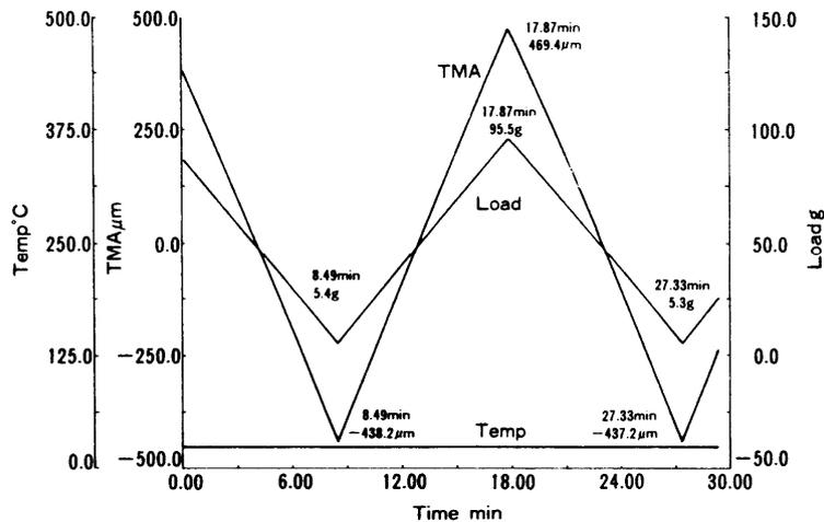
Figure 1 TMA/SS measurement results for spring
