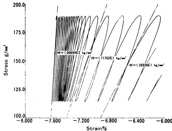
Figure 8 Stress-Strain graph for LDPE film (heating process)
