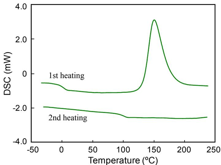
Figure 5 DSC curves of Carbon fiber reinforced epoxy prepreg
