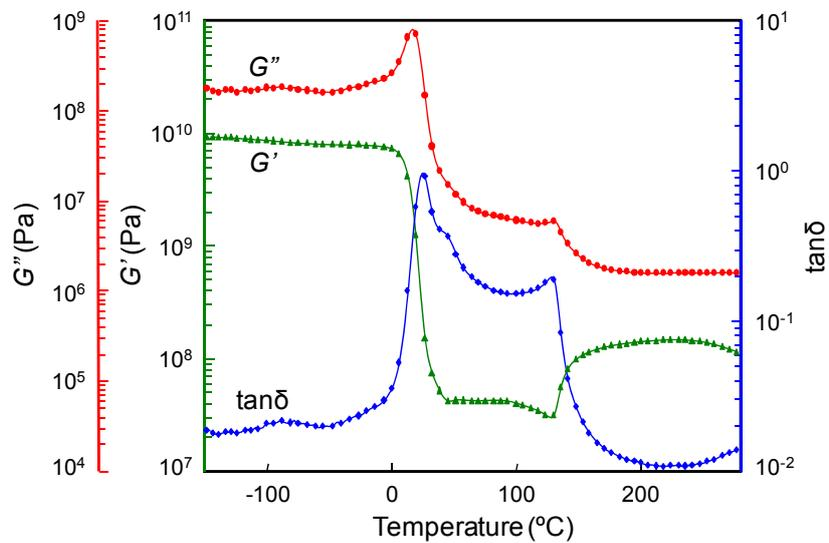
Figure 2 Viscoelastic spectrum of Carbon fiber reinforced epoxy prepreg (1st heating)
