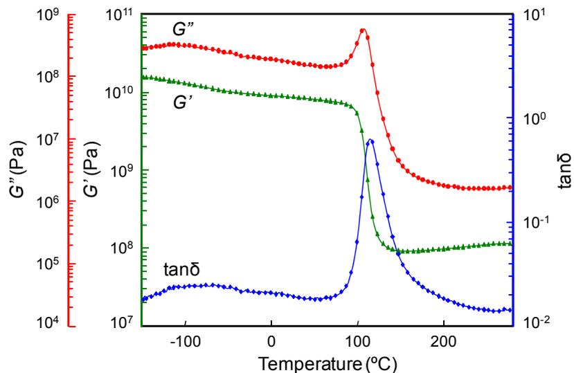
Figure 3 Viscoelastic spectrum of Carbon fiber reinforced epoxy prepreg (2nd heating)
