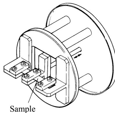
Figure 1 Film shear measurement head
