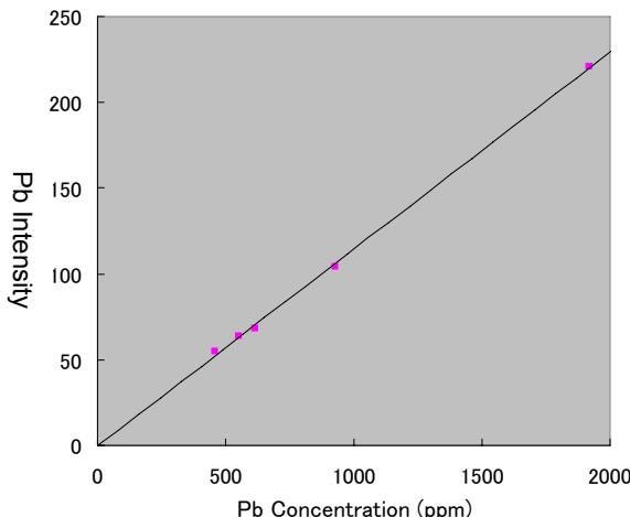
From the calibration curve, we calculated the lower detection limit and quantitative limit for Pb at 300 seconds of measurement. Based on the background inferred from each 74X HB spectrum, the lower detection limits and quantitative limit were defined as an intensity of three and ten times the theoretical statistical fluctuation, respectively. The lower detection limit for Pb was 7.9 ppm and the quantitative limit was 26.3 ppm.
