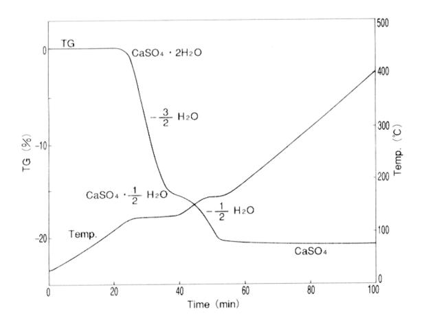
The above diagram shows a measurement data of Quasi-Isothermal Analysis (QIA), measuring calcium sulfate dihydrate (dihydrate gypsum) using QIA. Water evaporate from calcium sulfate dihydrate according to the below steps.
