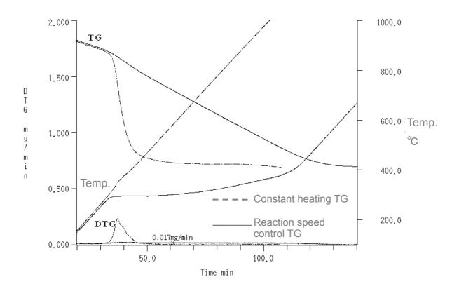
The above shows a measurement example of reaction speed control TG.
