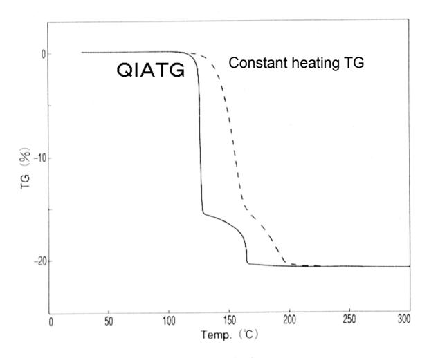
The above shows a data comparison between QIATG and constant heating TG. Taking the data from the previous page, the temperature axis is represented on the horizontal axis, and was compared to constant heating TG.
