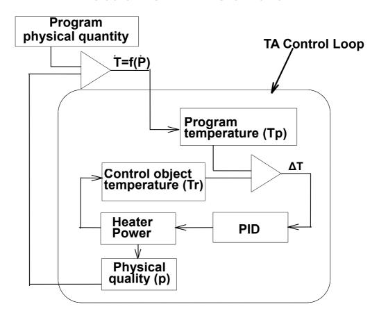
The above diagram shows an actually used CRTA control loop.
