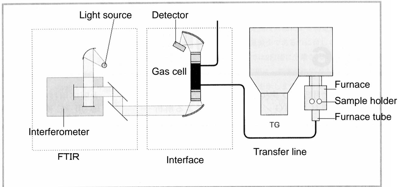
The above diagram shows an example of a TG/FT-IR system structure.
