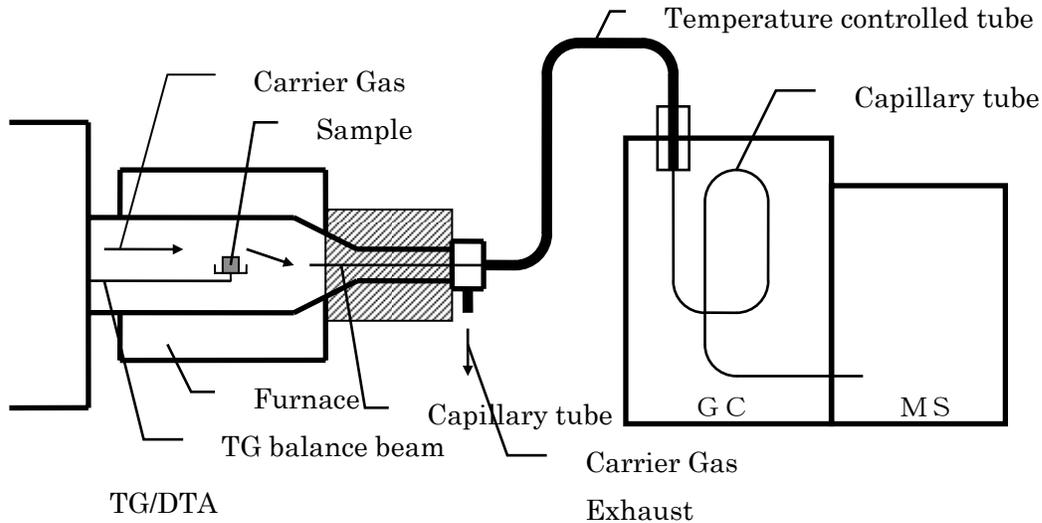
The above shows an example of a TG/MS system structure.
