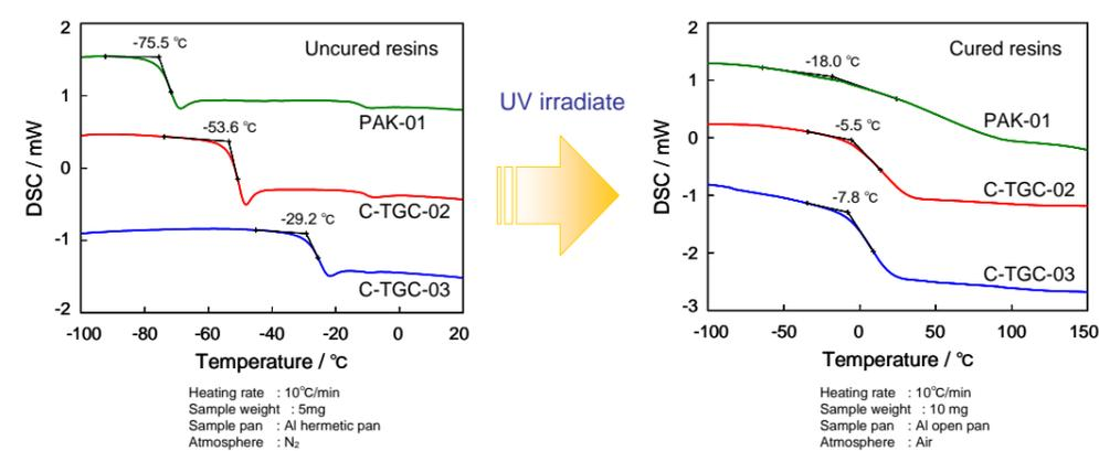
In case of same molecular structure polymer, the smaller the molecular weight, the lower the glass transition temperature becomes. Uncured resin, i.e. monomer, glass transition temperature is dependent on the amount of functional group equivalent. However as cured resin is already polymerized, the bigger the molecular weight by polymerization, the bigger the glass transition temperature difference might be.
