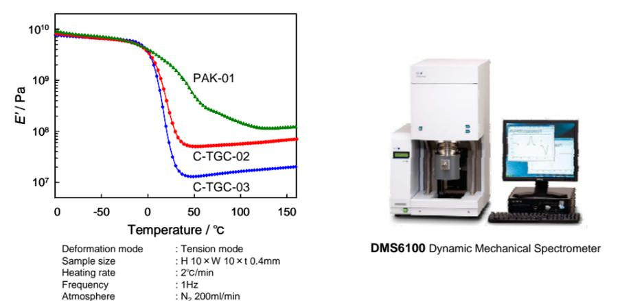
In case of cross-linked polymer, E' of the rubbery plateau region is detected higher the higher the crosslink density. Figure shows the smaller amount of functional group equivalent, the higher the crosslink density. It suggests that the resins which have smaller amount of functional group equivalent have small influence on the effect of steric hindrance and the effective polymerization.
