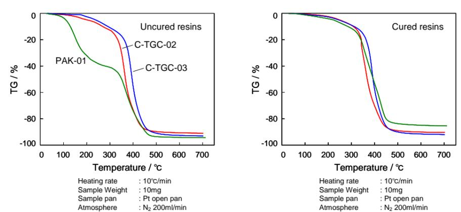
The higher amount of functional group equivalent, the higher decomposition temperature of both uncured resin and cured resin becomes. In particular, as C-TGC-3 contains phenyl in main chain, the highest decomposition temperature is likely to be obtained.
