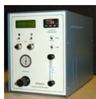
An example of humidity generator (InstruQuest Inc.)
