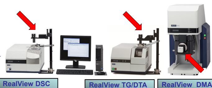
Fig.1 Thermal analyzers with optical observation units (red arrows) by Hitachi High-Tech Science Corp.
