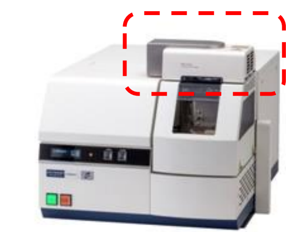
STA system with sample observation unit
