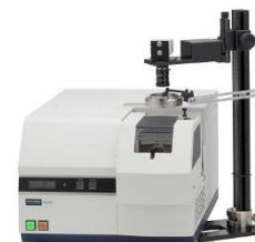
Thermo Gravimetry/ Differential Thermal Analyzer with Optical Observation Function STA7220
