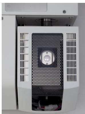
Furnace with sample viewing port
