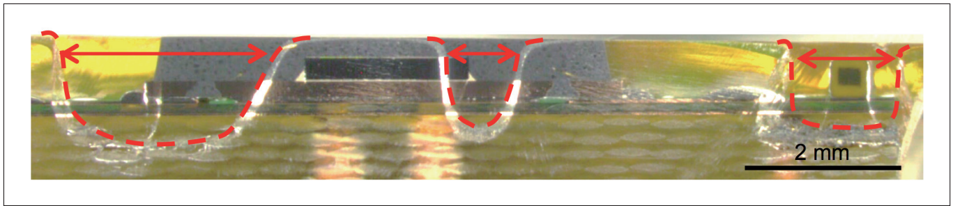
Fig. 9 Optical microscopy image of electronic circuit board sample prepared for observation using multi-site processing capabilities of ACS.
