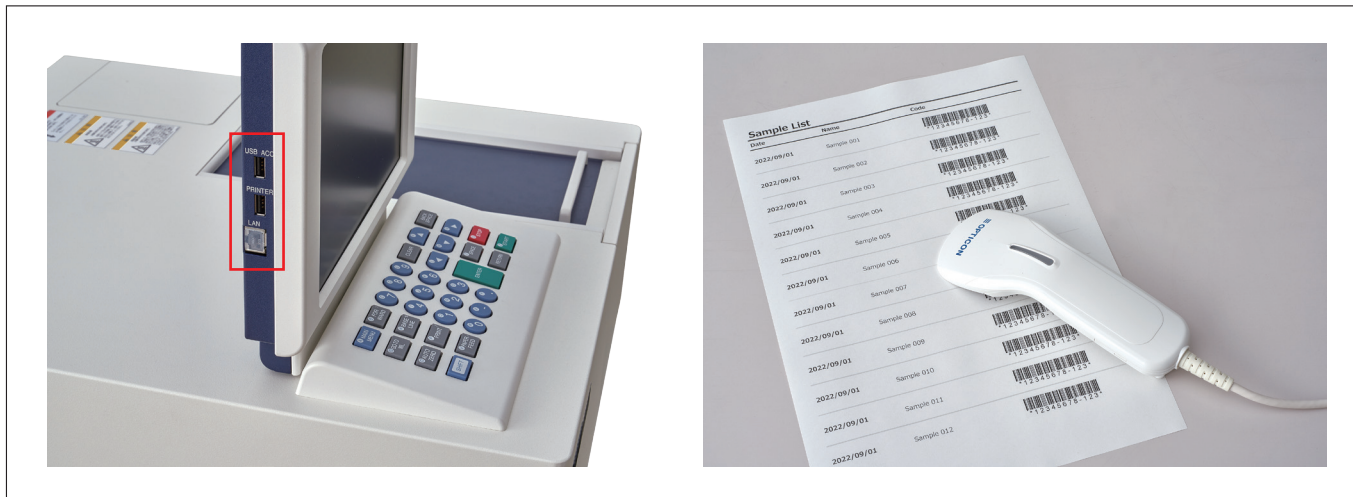
Fig. 6 UH5200-series instruments provide USB ports (left) for connecting external devices such as bar-code readers (right).
