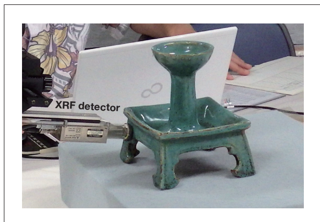
Fig. 17 Measuring X-ray fluorescence spectra for cultural property deemed a Japanese national treasure: square-base candle stand with green Ryoku-Yu glaze.
