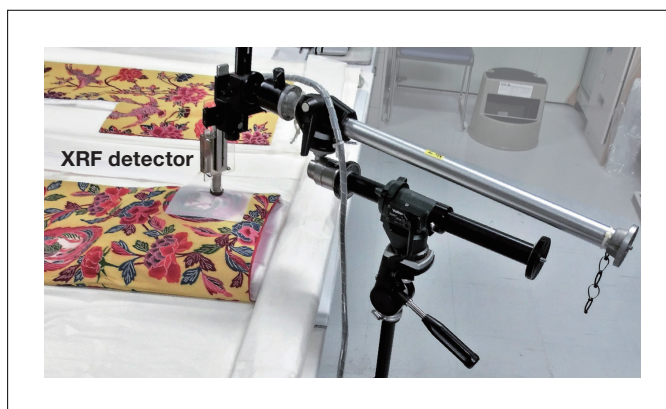
Fig. 16 Measuring XRF spectra for bingata specimen.
