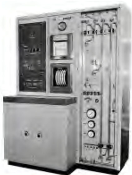
Complete automation of amino acid analysis: KLA-2
