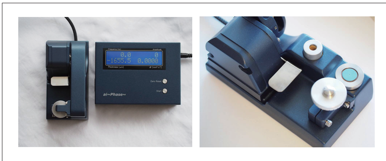
Fig 1. ai-Phase Mobile (Thin-film / thermal-diffusivity measurement model)
