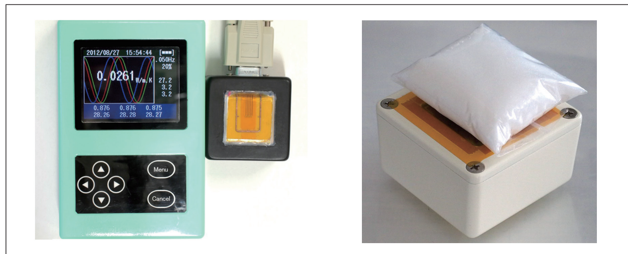
Fig 5. Full ai-Phase mobile instrument (bulk materials / thermal conductivity measurement model) and measurement of bagged powder sample
