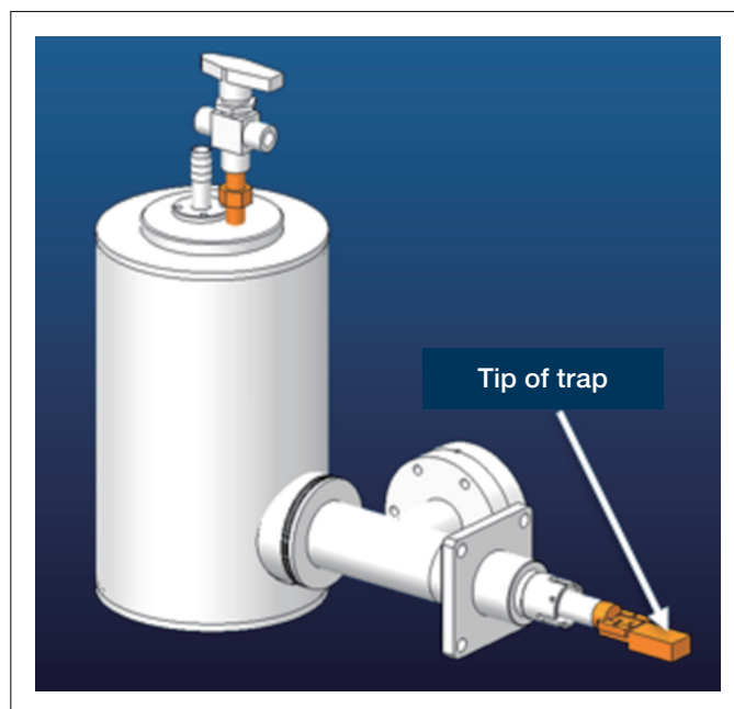
Fig. 2 CAD diagram of anti-contamination trap. The use of slush nitrogen succeeded in cooling to -200^{\circ}\text{C} . The shape of the tip of the trap was designed to surround the tip of the sample holder (the sample region).
