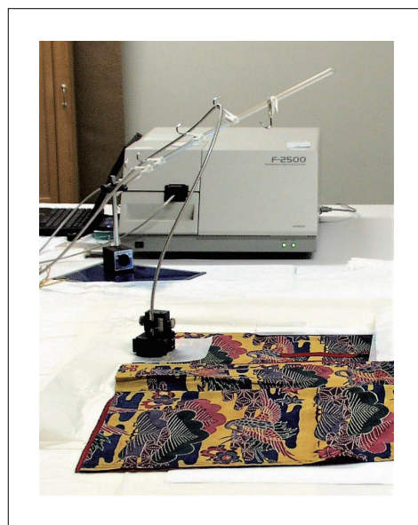
Fig. 25 Measuring 3DF spectra of bingata specimen.
