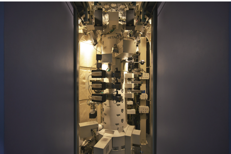
The 1 MV holography electron microscope. Akira Tonomura scoured Japan to find a site with the optimal geology and environment for this instrument, and eventually settled on its current location, Hatoyama. The instrument was built on a foundation of extremely hard ground rock.
