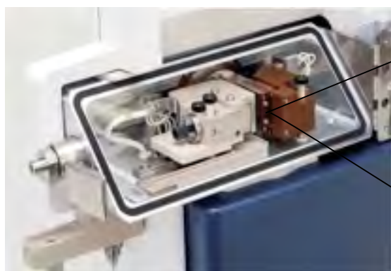
Fig.3 The interior of the ion source.
