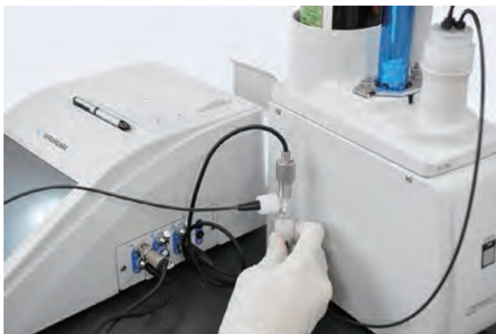
Fig. 2 Instrument with a titrant temperature sensor.
