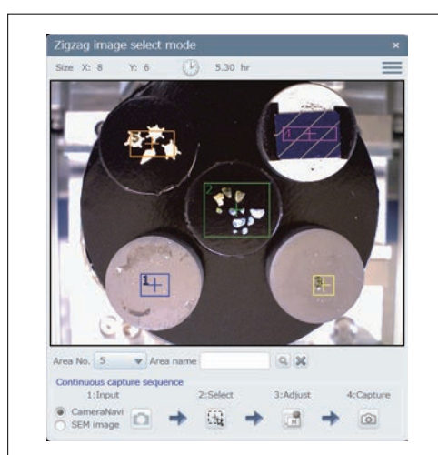
Fig. 4 Using Multi Zigzag to specify multiple sample regions.
