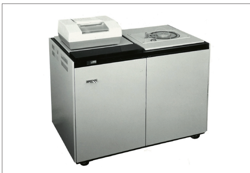
Fig. 1 Hitachi's Model 835 high-speed amino acid analyzer (1977). Whereas previous amino acid analyzers had been tall, the Model 835 was able to achieve a shorter footprint—for a reason.
