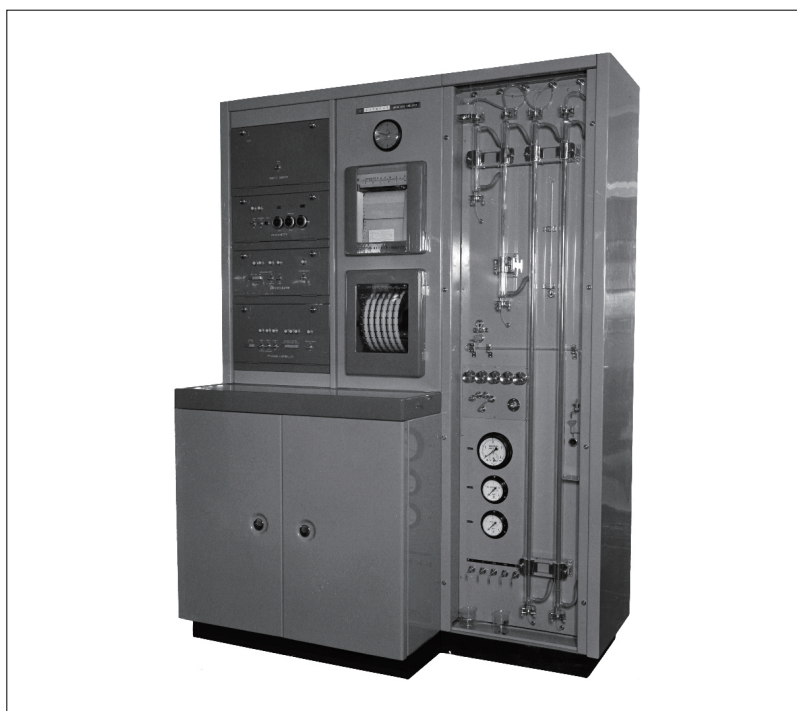
Fig. 4 The KLA-2 amino acid analyzer (1962). The long columns were made of glass and positioned vertically on the front instrument panel to allow their contents to be seen.
