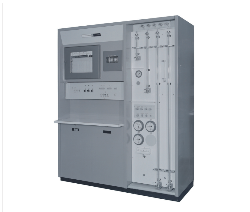
Fig. 3 Hitachi's KLA-3 amino acid analyzer, which was exported to countries including the Soviet Union, the U.S., and China.
