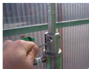
5. Loosen the flowmeter setscrew.
