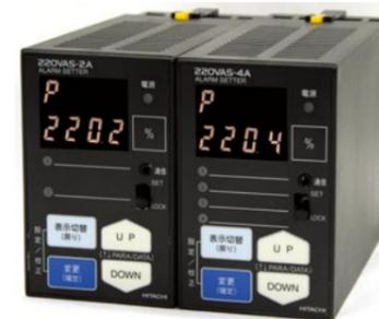
The alarms receive 4–20 mADC/1–5 VDC analog signals, compare them with the signals set in the units, and output alarm signals from up to four isolated relay contact points.
