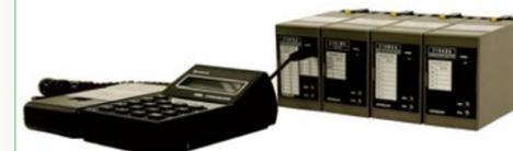
The compact plug-in type units receive signals from up to three points, execute a specified operation, and output the appropriate signals. The computing parameters are programmable using the model CMU-1 communicator.
