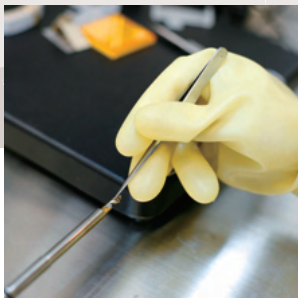
Putting a sample on the holder of electron microscope
