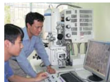
Dr. Minh and a researcher of IMS, operating SEM of Hitachi High-Technologies
