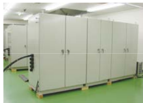
External appearance of the CP-2000P PCB monitor. The front hose takes in gas from the test facility for measurements.
