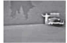
Image of car ahead as seen by an automotive night vision camera
